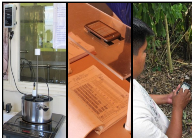
Figure 2: Examples of ODK tools in action. Left: Using Sensors to monitor breast milk pasteurization that deactivates contaminants (e.g. HIV virus); Center: Using Scan to digitize paper based vaccine information in Mozambique; Right: Indigenous tribal member using Collect in the Amazon jungle.
